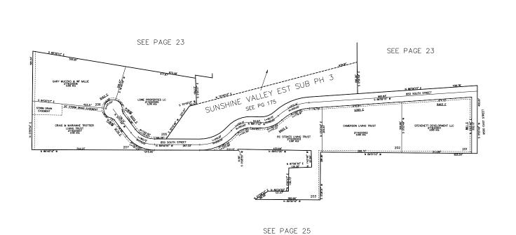
10' UTILITY & DRAINAGE EASEMENTS EACH SIDE OF PROPERTY LINES AS INDICATED BY DASHED LINES EXCEPT AS OTHERWISE SHOWN.
